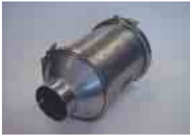
A Diesel Particulate Trap for reducing emissions, photo courtesy of SCAQMD.
